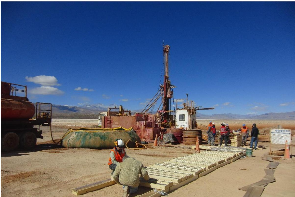
**Figure 2: Exploration Diamond Core Holes – Major Drilling**
