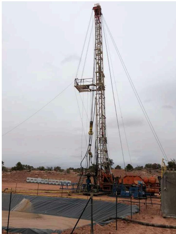
Figure 1: The work over rig at Gold Bar Unit 2, with bulk sample containers in the background.
