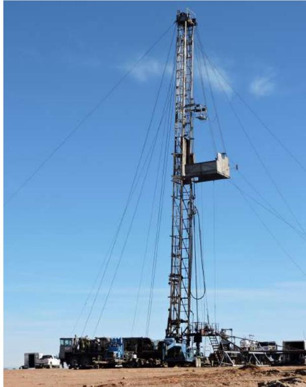
**Figure 2: photo of a work over rig.**
